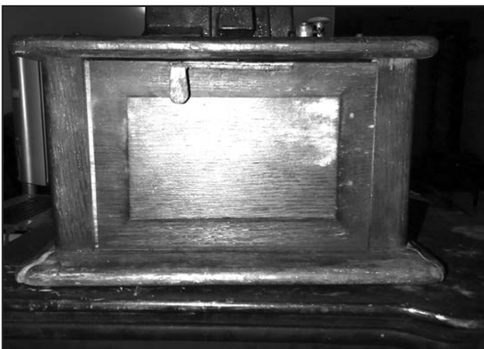
Showing the damage to the Triumph's case after I was unable to close it properly. Note the gap between the side and back plates.
